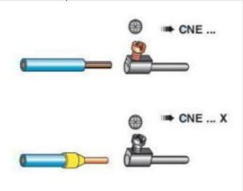
CNE ... X : for conductors with bush terminal
